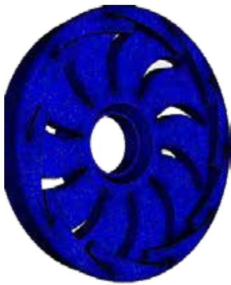
Model meshed with ~ 2 million elements
