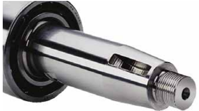
The tapered shaft and woodruff key design allow easy removal of the impeller from the rotating assembly.
