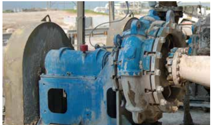
Model 5500 pumping Phosphogypsum in a phosphate plant.
