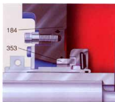
Slurry Mechanical Seal with Slurry Seal Chamber
