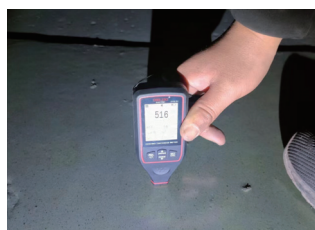
Anti-corrosion treatment of the inner surface of the bottom plate and side plates of the gas holder
